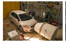
Chassis dyno for vehicle emissions testing
