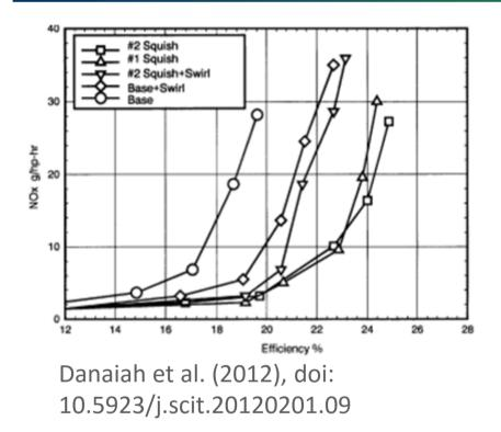
There is a **fundamental trade-off** between fuel consumption and NOx emissions (all engines - not only diesel)
